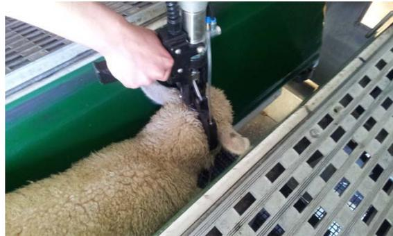
The end of the cycle is shown by the opening of the electrodes, thereby releasing the animals head. It is important that the trigger and remote safety switch remain constantly engaged until the cycle ends. An early release of the trigger and or remote safety switch results in a poor stun and or double stun.
